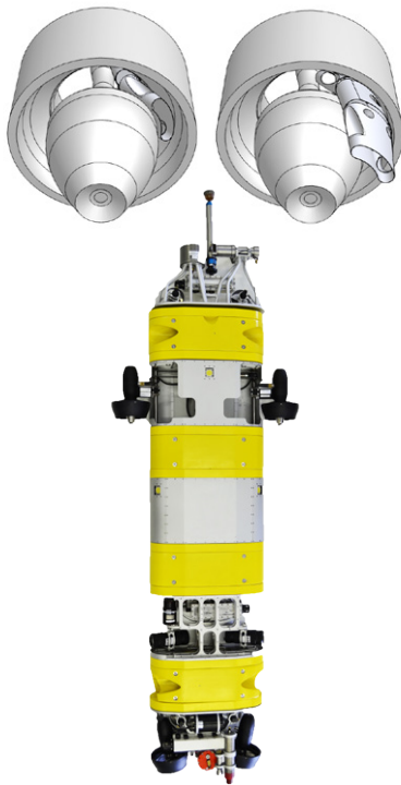
The flexible Chiton ROV can pass through curved structures, and then become rigid to move through the water by using hydraulics to control a series of ligaments.
