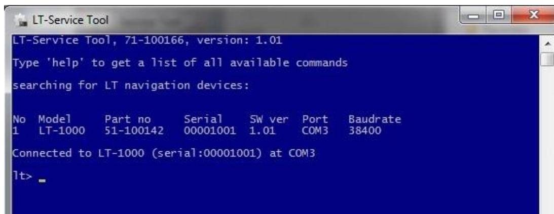
FIGURE 43: THE LT-SERVICE TOOL WILL AUTOMATICALLY SEARCH FOR LT-NAVIGATION DEVICES, WHICH ARE CONNECTED TO THE PC. A MANUAL CONNECTION MODE IS ALSO AVAILABLE.
