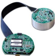
KVH's DSP-1750 FOG is the smallest high-performance fiber optic gyro in the world. The DSP-1750 FOG uses KVH's unique 170-micron E-Core ThinFiber, the smallest D-shaped optical fiber which is capable of delivering extremely low noise with very high bandwidth.
